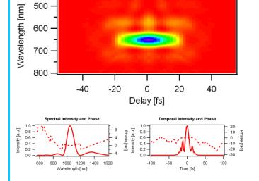
It shows a typical FROG trace. The pulse is from a fiber laser and the center wavelength is 1050nm. The pulse is suffering from a couple of chirp. After retrieving it, the program shows the temporal intensity and phase, and the spectral intensity and phase.
