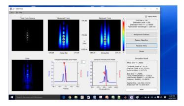
On the left, the model AFT-1550SFS is shown. The fiber coupler is an option for any model in the wavelength. On the right, the picture shows retrieving a double pulse by AFT SHG FROG software. Even though the pulse is complicated, the results are good. The center wavelength is 1550nm.
